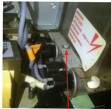
Remove 1/4" (7 mm) Hex Head Screw (Figure 12)
